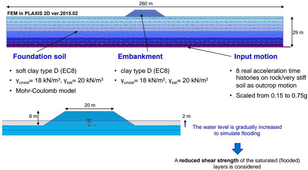
Figure 4. Numerical model in Plaxis 2D for SoA1: roadway/railway embankment and foundation soil, subjected to flood and seismic excitation
