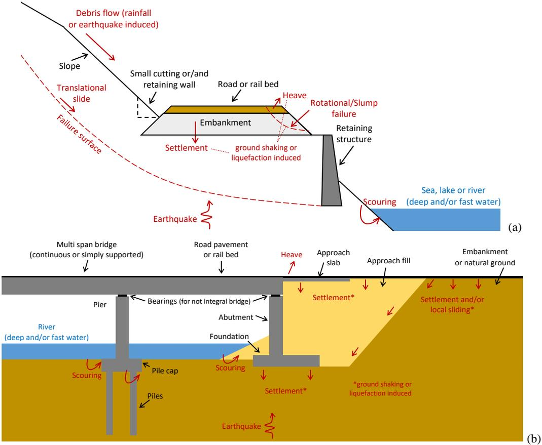
Figure 3. Multiple hazard effects on representative transport System of Assets: (a) embankment, slope, retaining structure (SoA1), (b) bridge, abutment, foundations, backfill (SoA2) (Argyroudis et al. 2019a).
