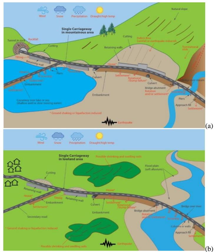
Figure 2. Transport infrastructure in diverse ecosystems exposed to multiple hazards: Lower capacity and speed roads (e.g. single carriageways) in (a) mountainous areas, (b) lowland areas (Argyroudis et al. 2019a).
