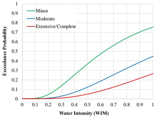
$WIM = \frac{h_{emb} - h_w}{h_{emb}}$ , WIM is the Water Intensity Measure,  $h_{emb}$  is the height of embankment,  $h_w$  is the depth to the groundwater table
