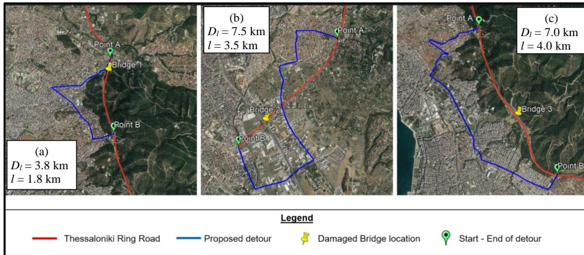
Figure 24. Alternative detours for (a) Bridge 1, (b) Bridge 2 and (c) Bridge 3.  $D_I$  is the detour length (blue line) and  $l$  is the length of the link (distance from point A to B on the red line).
