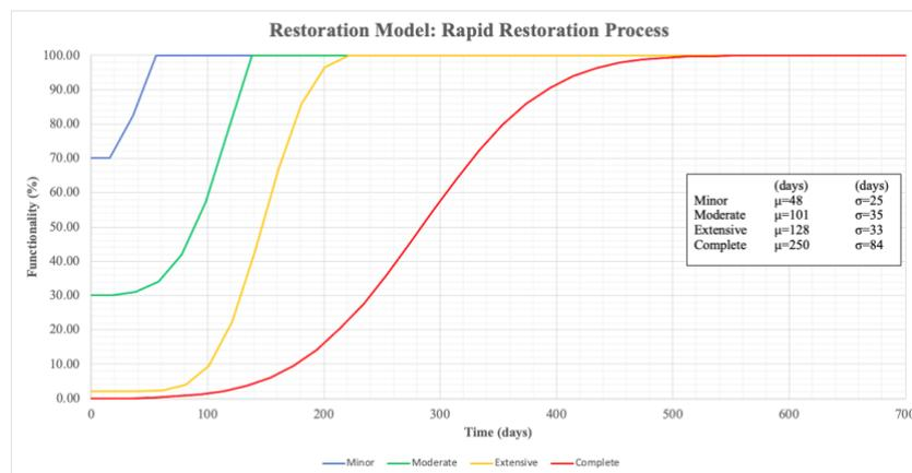
Figure 20. Example of restoration curves for hydraulic induced damage to spread foundations
