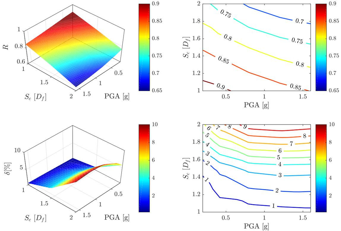
Figure 23. Behaviour of the resilience index,  $\mu_R$ , (plots at the top) and the coefficient of variation,  $\delta$ , (plots at the bottom) as a function of the scour (Sc) and the shaking level (PGA) (Argyroudis et al. 2020a).
