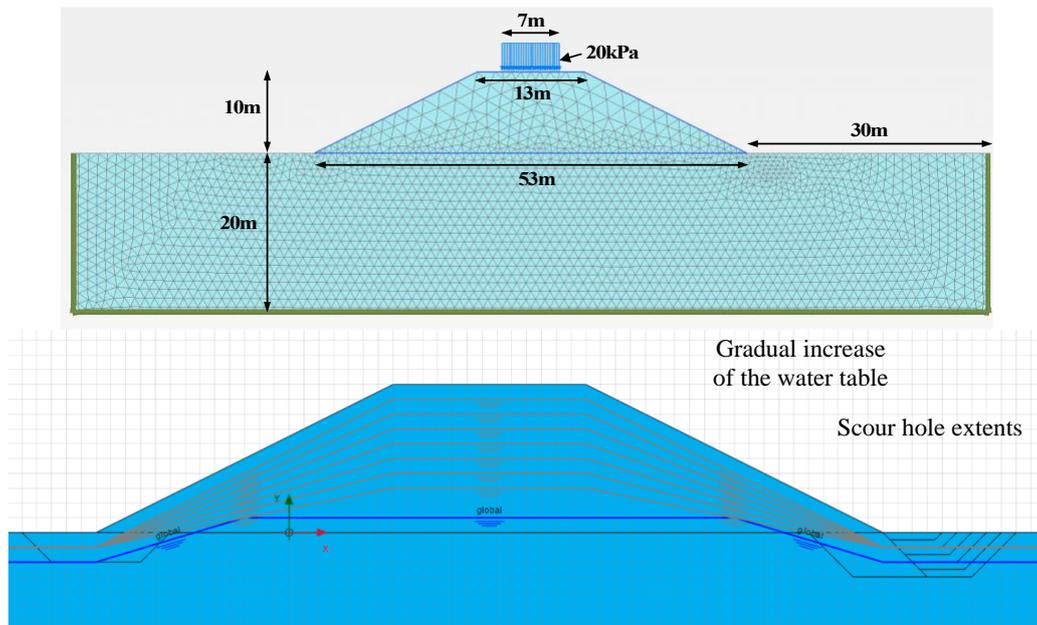
Figure 5. Numerical model in Plaxis 2D for SoA1: embankment and foundation soil, subjected to moisture ingress and scour effects
