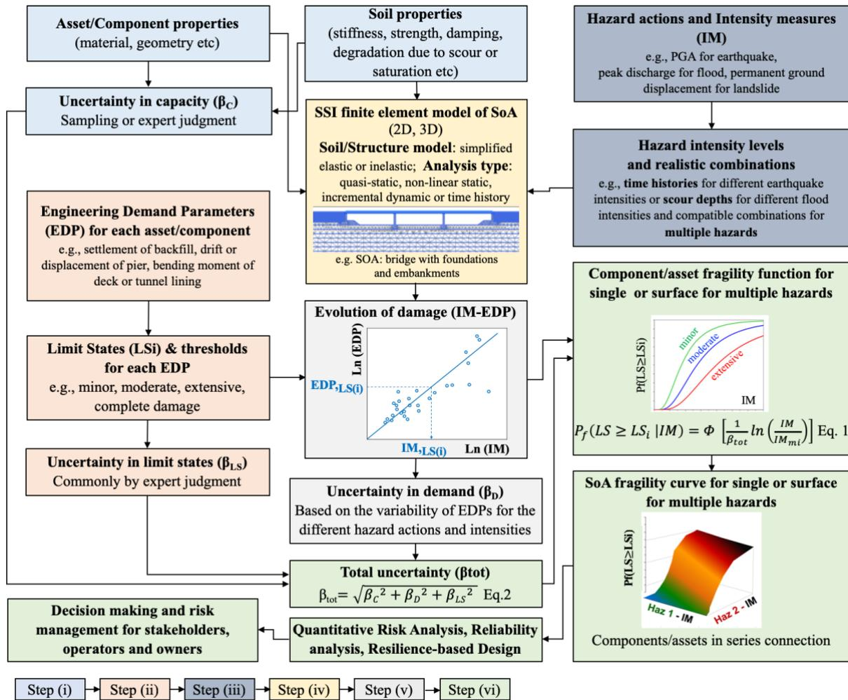
Figure 8. Flowchart for multiple hazard fragility functions of transport systems of assets (Argyroudis et al. 2019a).
