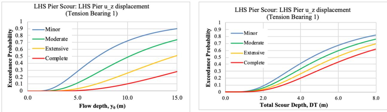
Figure 11. Examples of multiple hazard fragility functions for representative components of SoA2 (deck section, pier footing, abutment, bearings) exposed to flood, scour and debris accumulation effects, as a function of scour depth (right) and flow depth (left).
