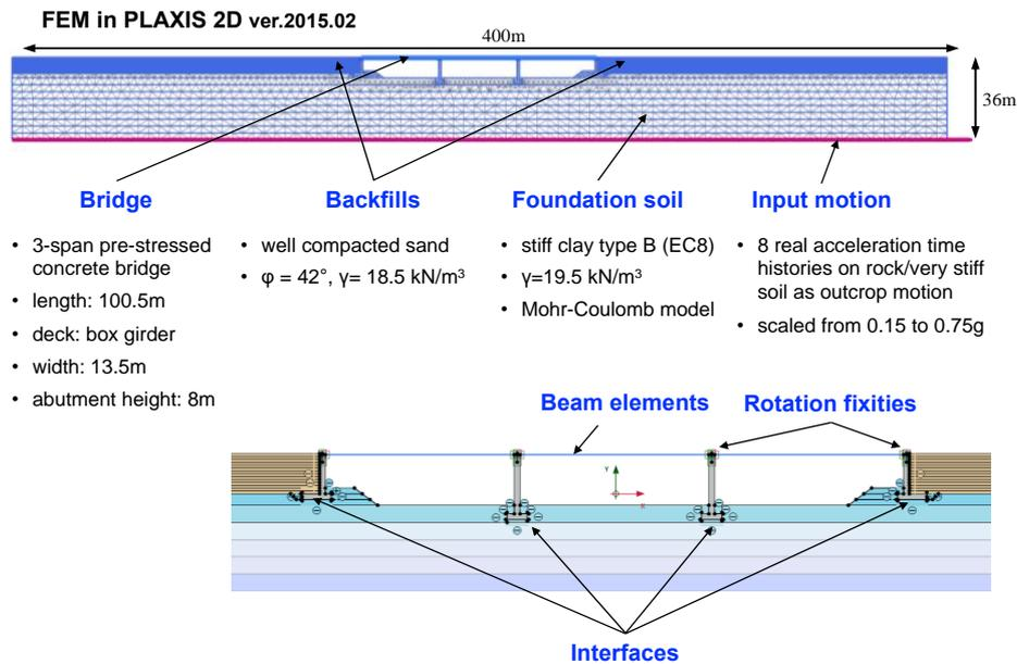
Figure 6. Numerical model in Plaxis 2D for SoA2: bridge, backfills, foundation soil subjected to seismic shaking
