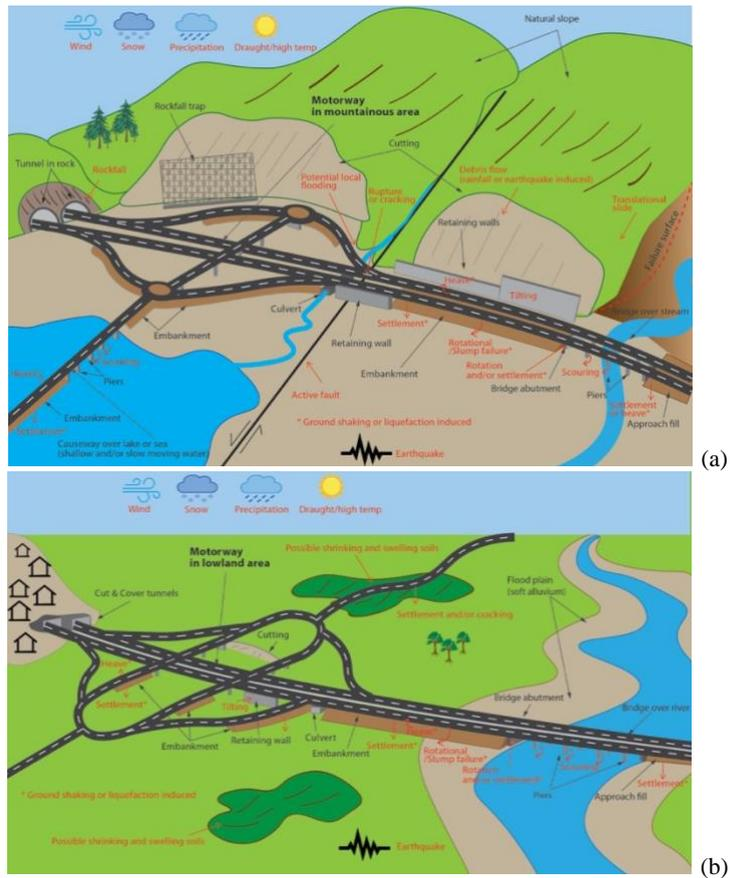
Figure 1. Transport infrastructure in diverse ecosystems exposed to multiple hazards: High capacity and speed roads (e.g. motorways) in (a) mountainous areas, (b) lowland areas (Argyroudis et al. 2019a).
