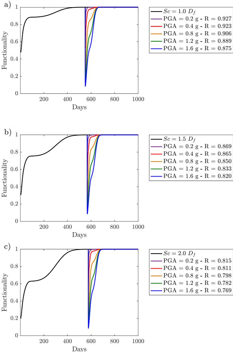
Figure 21. Resilience curves for the case that Haz-2 (EQ at PGA levels equal to 0.2, 0.4, 0.8, 1.2 and 1.6 g) occurs after the total recovery from Haz-1: a)  $Sc = 1.0D_f$ , b)  $Sc = 1.5D_f$ , and c)  $Sc = 2.0D_f$  (Argyroudis et al. 2020a).
