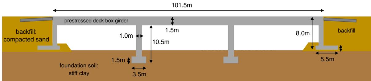
Figure 16. The 3-span prestressed concrete reference bridge
