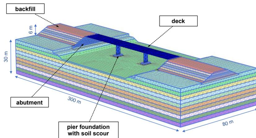
Figure 7. Numerical model in Plaxis 3D for SoA2: bridge, backfills, foundation soil, subjected to flood and scour effects
